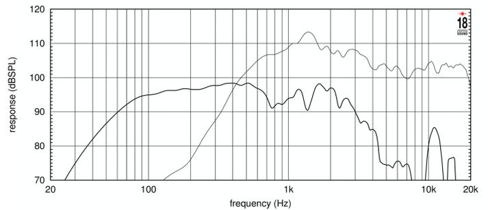
**MADE ON 125 LIT. ENCLOSURE TUNED AT 45 HZ IN FREE FIELD (4PI) ENVIRONMENT. ENCLOSURE CLOSES THE REAR OF THE DRIVER. THE THIN LINE REPRESENTS THE HIGH FREQUENCY RESPONSE. FREE AIR IMPEDANCE MAGNITUDE CURVE**
