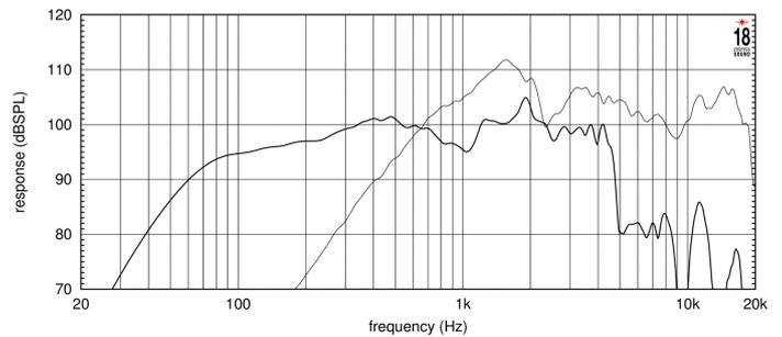
**FREQUENCY RESPONSE CURVE MADE ON 125 LT ENCLOSURE TUNED 50HZ IN FREE FIELD (4PI) ENVIRONMENT. ENCLOSURE CLOSES THE REAR OF THE DRIVER. THIN LINE REPRESENTS HIGH FREQUENCY RESPONSE. FREE AIR IMPEDANCE MAGNITUDE CURVE**
