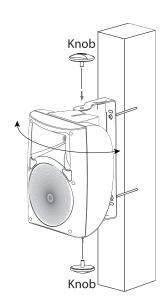
Attach the speakers to the brackets, lightly screw the bracket knobs into the cabinet and Point the speaker toward the listening area. Once the direction of the speaker has been determined tighten the bracket knobs securely.
