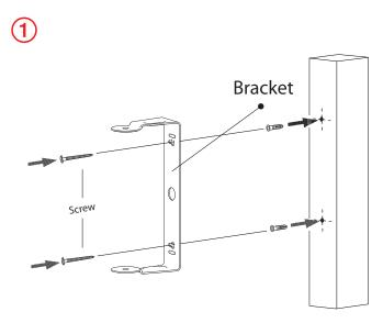
Using the bracket supplied, first make location and placement and then mount the bracket. For safety reasons do not mount a speaker on a wall made of unreinforced drywall or plasterboard. If you are not sure consult a professional installer.
