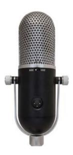
The Heil PR 77 D features a two-position switch allowing the selection of the best characteristics for voice or music. The voice position rolls the audio off at 120 Hz at -6 dB per octave while the music selection removes the filter and the entire audio spectrum of 60 Hz to 16 kHz is present.
