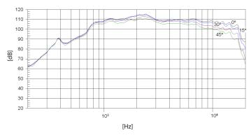
**Note:** dispersion measured with two waveguides coupled to TD-WL4 horn in anechoic chamber, 1W @ 1m.
