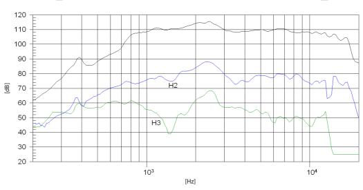
Note: On axis frequency response measured with two waveguides coupled to TD-WL4 horn in anechoic chamber, 1W @ 1m
