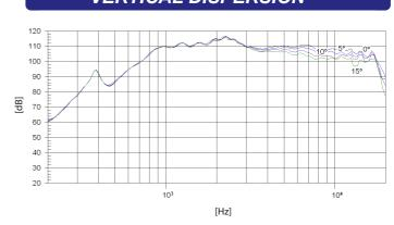
Note: dispersion measured with two waveguides coupled to TD-WL4 horn in anechoic chamber, 1W @ 1m.
