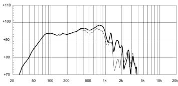
FREQUENCY RESPONSE CURVE OF 15NLW9500 MADE ON 180 LIT. ENCLOSURE TUNED AT 35HZ IN FREE FIELD (4PI) ENVIRONMENT. ENCLOSURE CLOSES THE REAR OF THE DRIVER. THE THIN LINE REPRESENTS 45 DEG. OFF AXIS FREQUENCY RESPONSE.
