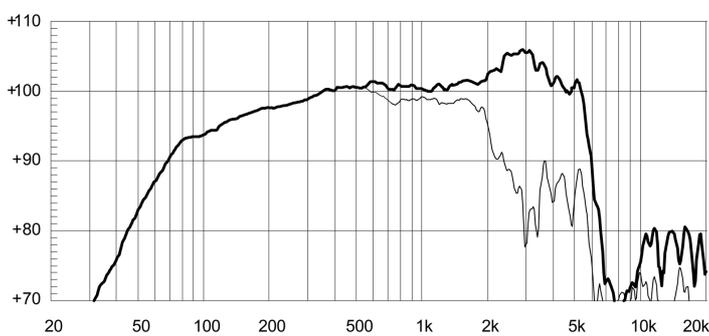
**FREQUENCY RESPONSE CURVE OF 12NMB420 MADE ON 18 LIT. ENCLOSURE TUNED 60HZ IN FREE FIELD (4PI) ENVIRONMENT. ENCLOSURE CLOSES THE REAR OF THE DRIVER. THE THIN LINE REPRESENTS 45 DEG. OFF AXIS FREQUENCY RESPONSE**
