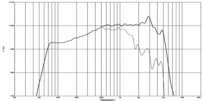
**FREQUENCY RESPONSE CURVE OF 10NMB420 MADE ON 30LIT. ENCLOSURE TUNED @ 55HZ IN FREE FIELD (4PI) ENVIRONMENT. ENCLOSURE CLOSES THE REAR OF THE DRIVER. THE THIN LINE REPRESENTS 45 DEG. OFF AXIS FREQUENCY RESPONSE.**
