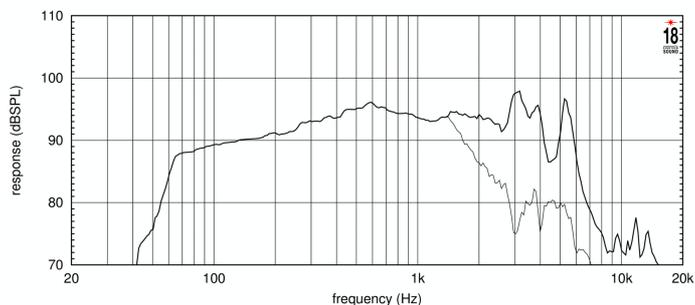
**FREQUENCY RESPONSE CURVE OF 8NW650 MADE ON 25LIT. ENCLOSURE TUNED 65HZ IN FREE FIELD (4PI) ENVIRONMENT. ENCLOSURE CLOSES THE REAR OF THE DRIVER. THE THIN LINE REPRESENTS 45 DEG. OFF AXIS FREQUENCY RESPONSE**
