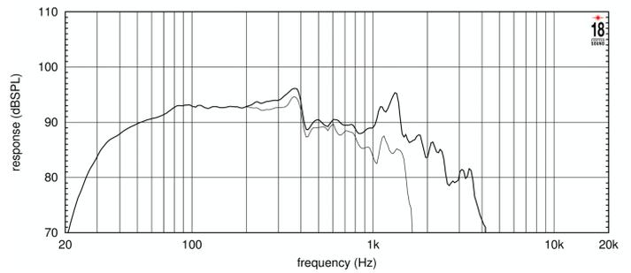
**FREQUENCY RESPONSE MADE IN 180 LT. ENCLOSURE TUNED AT 35 Hz IN FREE FIELD (4p) ENVIRONMENT. ENCLOSURE CLOSES THE REAR OF THE DRIVER, THE THIN LINE REPRESENTS 45° OFF AXIS FREQUENCY RESPONSE FREE AIR IMPEDANCE MAGNITUDE CURVE**
