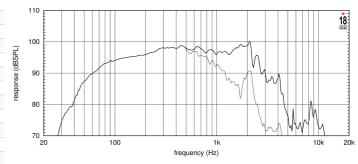
FREQUENCY RESPONSE CURVE MADE ON 125 LIT. ENCLOSURE TUNED 50HZ IN FREE FIELD (4PI) ENVIRONMENT. ENCLOSURE CLOSES THE REAR OF THE DRIVER. THE THIN LINE REPRESENTS 45 DEG. OFF AXIS FREQUENCY RESPONSE FREE AIR IMPEDANCE MAGNITUDE CURVE
