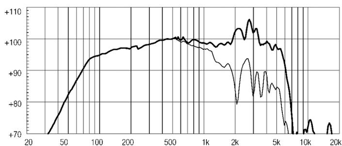
**FREQUENCY RESPONSE CURVE OF 12W500 MADE ON 50 LIT. ENCLOSURE TUNED 60HZ IN FREE FIELD (4PI) ENVIRONMENT. ENCLOSURE CLOSES THE REAR OF THE DRIVER. THE THIN LINE REPRESENTS 45 DEG. OFF AXIS FREQUENCY RESPONSE**
