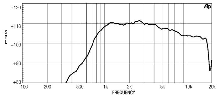
**ND1090 MEASURED WITH 1W INPUT ON RATED IMPEDANCE AT 1M DISTANCE ON XT1086 HORN MOUTH AXIS FREE AIR IMPEDANCE MAGNITUDE CURVE**
