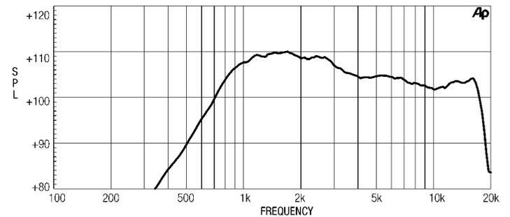
**HD1040 MEASURED WITH 1W INPUT ON RATED IMPEDANCE AT 1M DISTANCE ON XT1086 HORN MOUTH AXIS FREE AIR IMPEDANCE MAGNITUDE CURVE**
