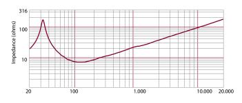
Frequency (Hz) Impedence magnitude curve measured in free air
