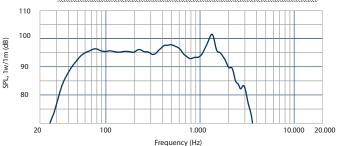
Frequency response curve of the loudspeaker make in a hemispherical, free field and mounted in a reflex box with an internal volume of 55 litres and tuned at 60Hz, applying a sinusoidal signal of 2.83 V @8 at 1m.
