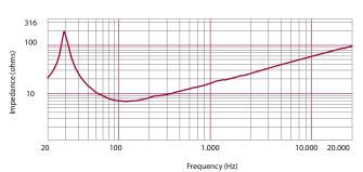
Impedence magnitude curve measured in free air
