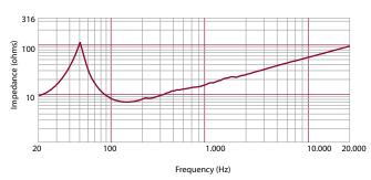
Impedence magnitude curve measured in free air
