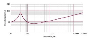
Impedence magnitude curve measured in free air
