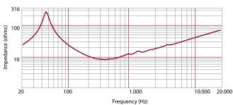
Impedence magnitude curve measured in free air
