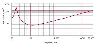
Impedence magnitude curve measured in free air
