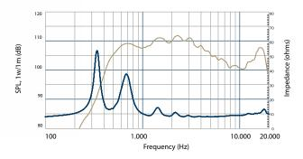
Frequency response and electrical impedance curve of the compression driver mounted on  $90^\circ\text{Hx}40^\circ\text{V}$  horn with input signal of 2.83 Volt
