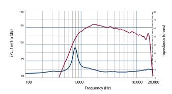
Frequency response and electrical impedance curve of the compression driver mounted on 90°Hx40°V horn with input signal of 2.83 Volt
