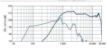
Frequency (Hz) Frequency response curve of the loudspeaker make in a hemispherical, free field and mounted in a reflex box with an internal volume of 50 litres and tuned at 60Hz, applying a sinusoidal signal of 2.83 V@8 at 1m.
