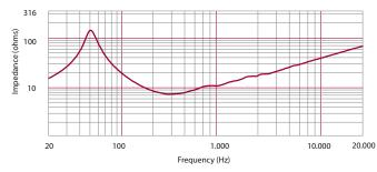
Impedence magnitude curve measured in free air
