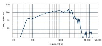
Frequency response curve of the loudspeaker make in a hemispherical, free field and mounted in a reflex box with an internal volume of 55 litres and tuned at 60Hz, applying a sinusoidal signal of 2.83 V @8 at 1m.
