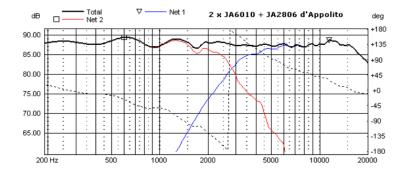
The smooth roll off characteristic provides easy filtering at points of crossover around 2-3 kHz. Example of d'Appolito setup with JA-2806 tweeter.
