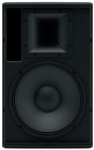
The X12 fulfils the requirement for a compact system that can deliver high sound levels — either as a stand-alone system or supplemented by a BlacklineX subwoofer. Featuring a 12" (300mm) LF driver unit and a 1" (25mm) exit compression driver on a user-rotatable horn, its  $80^{\circ}$  x  $50^{\circ}$  dispersion pattern is ideal for medium throw applications.
