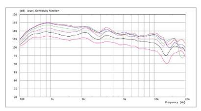
0/10/20/30/40/50 degree off-axis horizontal HF response (wide-axis).
