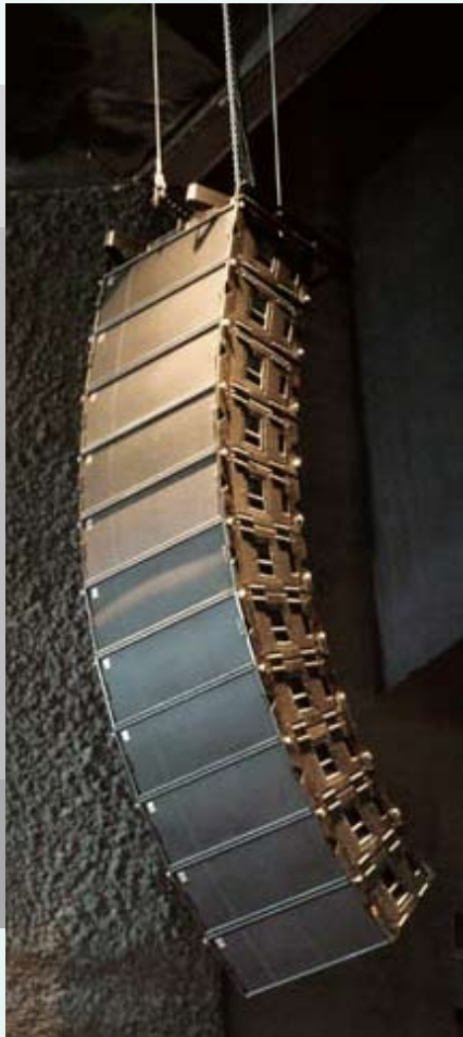
▲ Banana array is wasteful of array elements
