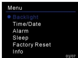
Select illuminated level of backlight (High/Medium/Low) and the duration of timeout (On/10/20/30/45/60/90/120/180 sec). With setting the timeout, the backlight will automatically change to dim if the device is not accessed for operation at the setting time.
