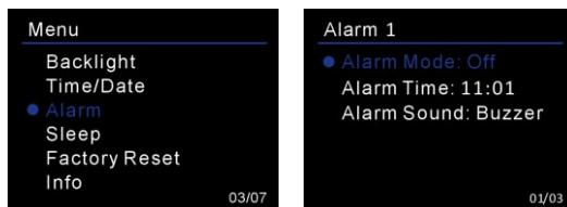
Rotate the < TUNING /SELECT> control to choose setting up Alarm 1 or Alarm 2. Press the < TUNING /SELECT> control to enter the detailed settings.
