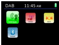
Press **MODE** button to go to the main menu, you can rotate the < **TUNING /SELECT**> control to select different operation mode (DAB, FM, AUX IN or Bluetooth) and then press the < **TUNING /SELECT**> control to confirm.
