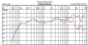
Extended frequency measure, 30 deg off axis in red
