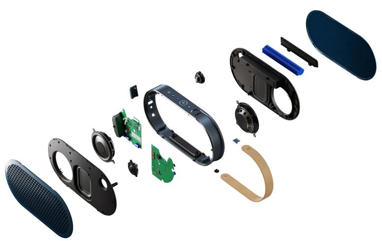
Placing drivers on both sides of the DALI KATCH helps the audio signal integrates with the entire room
