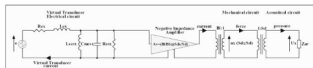
Figure 5 – Simplified model with a set of desired virtual parameters included before the Negative Impedance Voltage Buffer.
